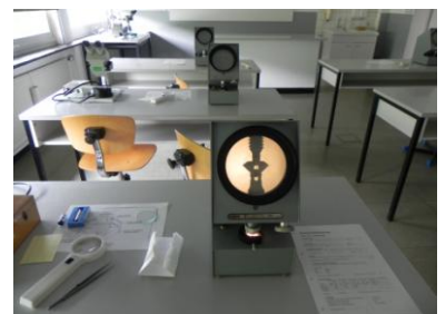
The proportion scope provides percentages based on the proportions and the symmetry of certain characteristics of round brilliant cut and modified brilliant cut diamonds.
